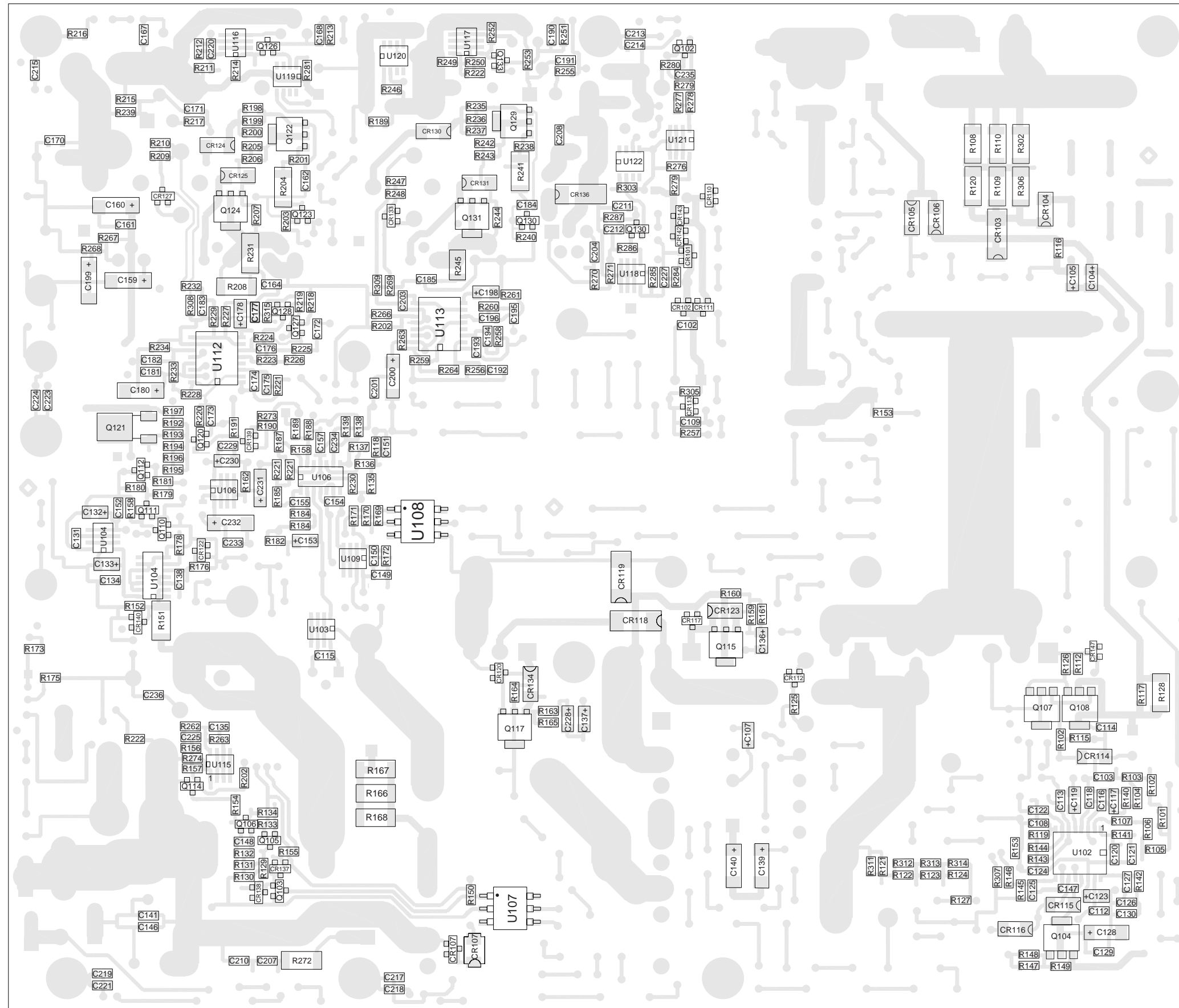
800W POWER SUPPLY COMPONENT LAYOUT (OPPOSITE COMPONENT SIDE VIEW) FIGURE10-44
